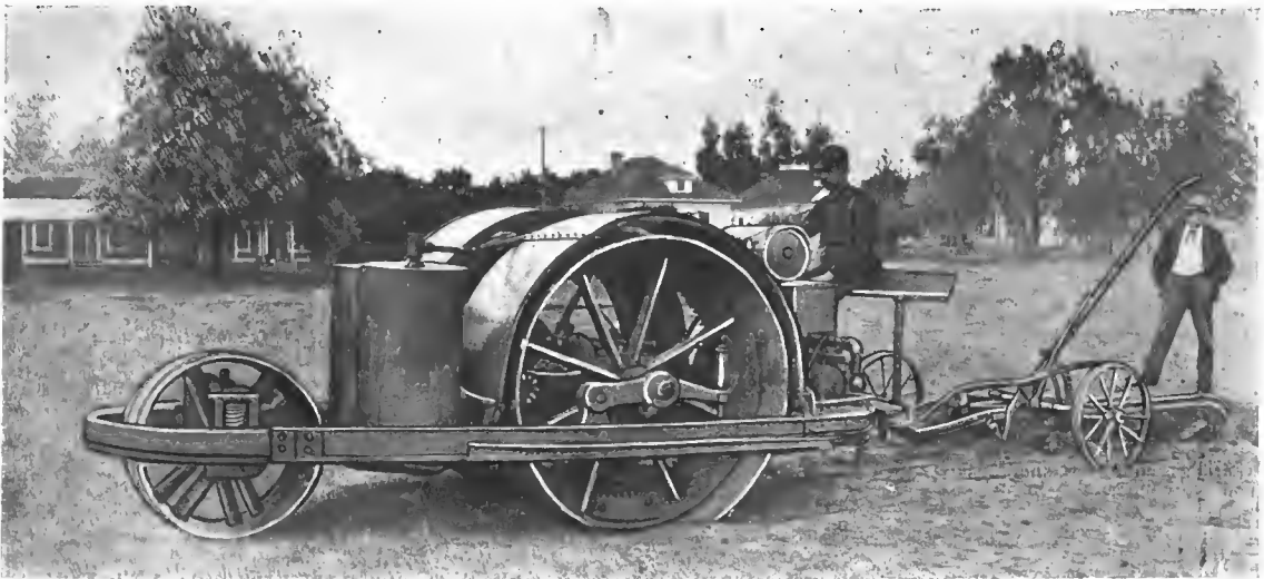
Plowing Six Furrows at One Operation with One of the Specially Designed Auto Farm Tractors, in California.
